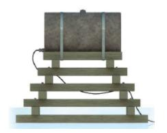
Elevate and strap fuel tanks above flood levels to prevent the tanks from floating away and causing more damage.
