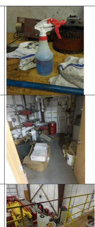
Secondary containers must be labeled to show any hazardous chemicals and comply with the new Hazard Communication Standard. 1910.1200(f)(6)
