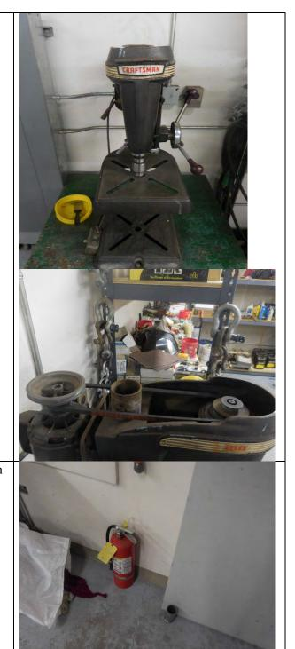
Extinguishers should be mounted on brackets or in wall cabinets with the carrying handle placed 3-1/2 to 5 feet above the floor. NFPA 10 6.3.1.1
