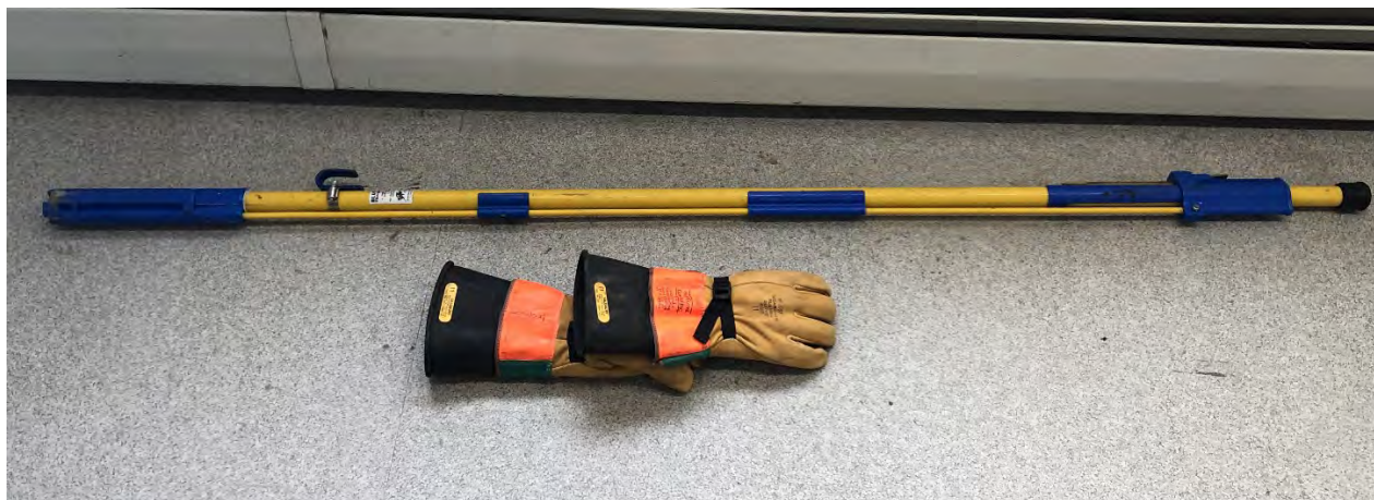
Example 1. Hot Stick and High Voltage Gloves
